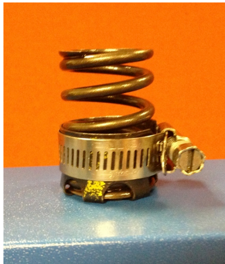
Figure 3: Image of VFD installed on Ford Spring
