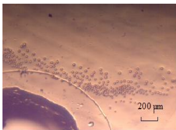
Figure 7: Photo showing sealing failure at inlet port, resulting in the leaking of sample fluid.
